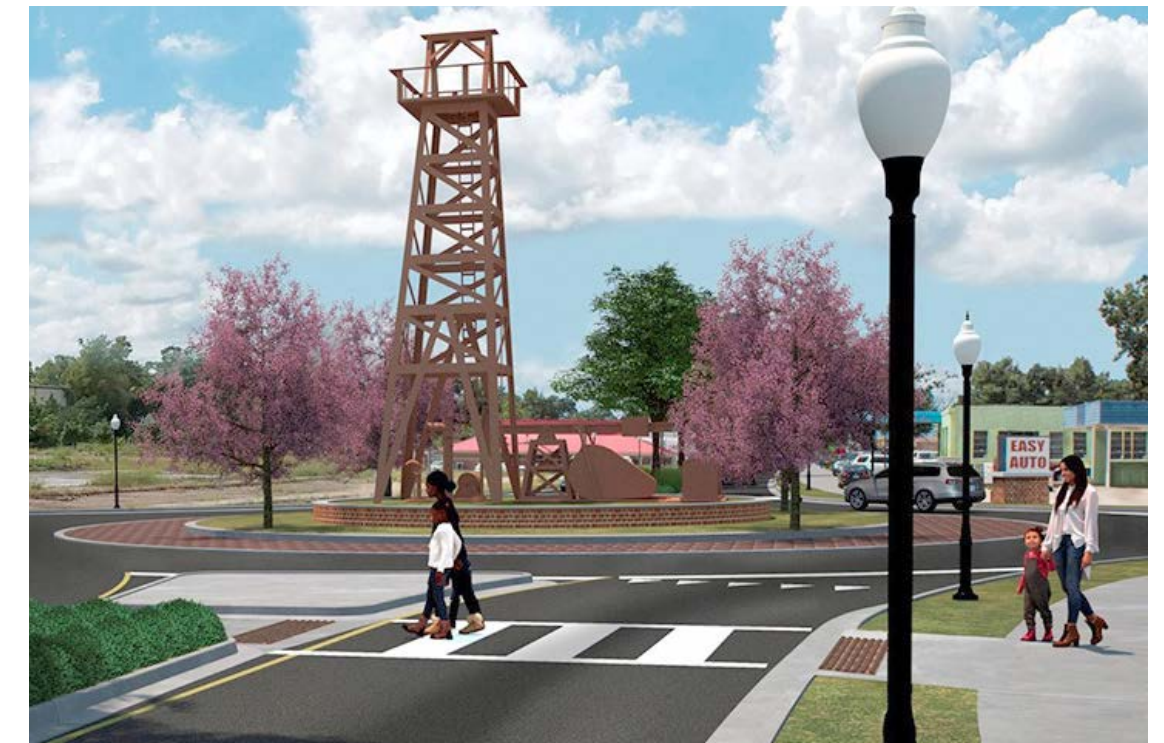
Roundabout illustration with features that could be utilized at Berlin Town Center. Note the landscape buffer, attractive human-scaled lighting, and continental-style crosswalk with side-lines. Source: Toole Design Group
