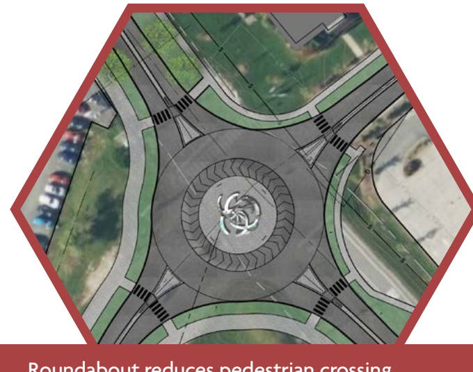
Roundabout reduces pedestrian crossing distances and reduces traffic congestion at intersection
